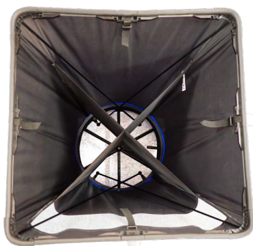
Hood with flow straightener
